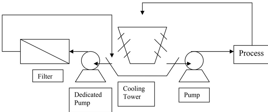
Figure 4. Side-stream Filtration with a Dedicated Pump
