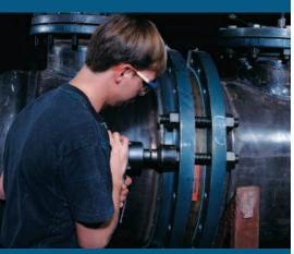
To ensure safety and optimal performance, all Thrush heat exchangers are constructed under an approved quality control program according to and registered with the National Board of Boiler and Pressure Vessel Inspectors. Additionally, each unit is manufactured, tested, and "U" stamped to ASME Code requirements under Section VIII Division 1, and a Manufacturer's Data Report for Pressure Vessels Form No. U-1 is provided with every unit.
