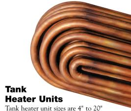
diameter unit sizes are 4" to 20" diameter with 24" to 120" lengths. Standard tank heaters are constructed in accordance to ASME requirements for the same pressure and temperature ratings as the "U" Tube Heat Exchangers. A Manufacturer's Data Report for Pressure Vessels Form No. U-1 is available upon request. All options available for "U" tube heat exchangers can be applied to tank heaters
